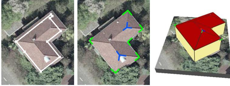
**Fig. 3.** A L-shaped building with its ground plan. In the ground plan additional details occur, which are not observable in the roof outline. Also a displacement due to roof overhangs is visible. The middle picture shows results of the eaves corners (green) and ridge corners (blue) extracted by our feature extraction (see section 5). The picture on the right shows our reconstruction result.
