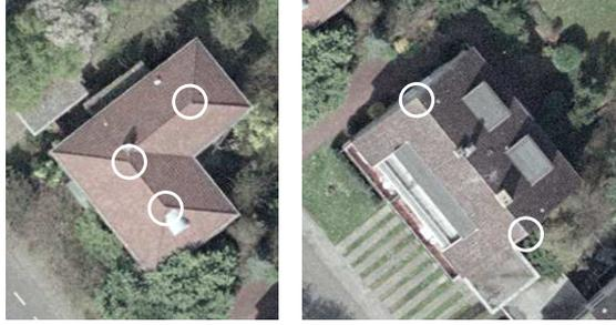
**Fig. 4.** The different types of ridge corners. The left figure shows the ridge corners, which results from intersection of inner roof edges. The second type of ridge corners is shown in the right figure.
